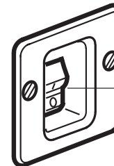
AC (Mains) Power Switch (Switch Guard not shown)
